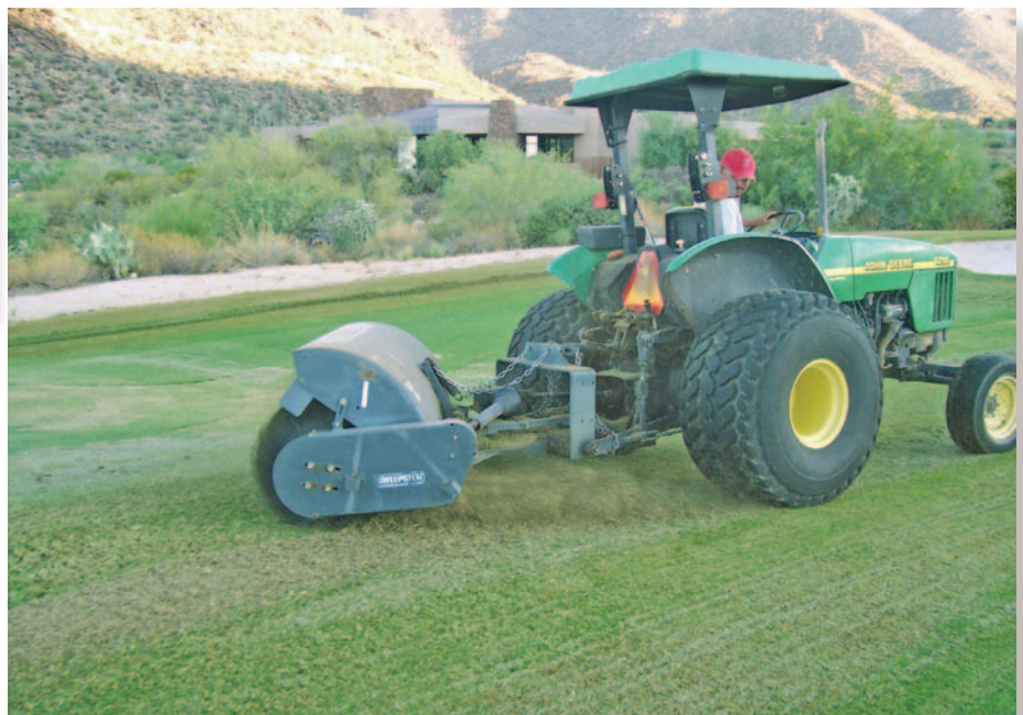
Figure 1. A power road broom removes ryegrass and plant debris, but causes minimal disturbance to bermudagrass.
